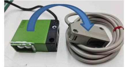
The kit M0620MS was developed to help fit the new style photocell into existing Gascoigne Melotte Tandem controllers. It may also be used when fitting components to a new enclosure. The original photocell was green and larger so some adaptation is needed to change to the smaller grey version.
